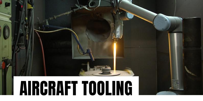
Aircraft Tooling Inc. (ATI) in Dallas, Texas is a repair center for the aviation industry, with processes including High Velocity Oxygen Fuel (HVOF) and plasma spray.
